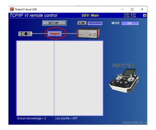
At this stage, the communication indicator reads **stopped** because the communication is not set up so far. It will start as soon as a controller software is started.
