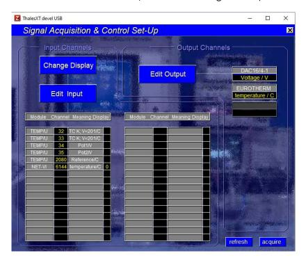
In this section, the Eurotherm (NET-VI, Channel:6144) will be used as an example of the external device and will be configured for use in the Thales Remote. First of all, the user must set up the Eurotherm as explained in the application note <u>Eurotherm</u>. Afterward, the user can use the command strings provided below to start the VI software (Eurotherm) and read the signal from channels in the Thales Signal Acquisition software.
