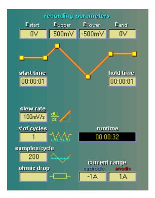
The parameters can easily be modified by entering the input page of the control parameters. The "recording parameters" section of the CV control panel comes up a little different if the optional ADF function is present in the case of the *Zennium-pro* or the *Zennium-X*.
