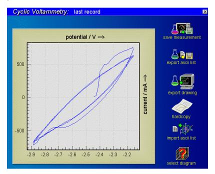
The CV curve measured (or loaded by file) last is displayed as shown above after the 'display diagram' has been entered. The data window is situated in the middle of the screen. On the right, five i/o standard interfaces offer transfer functions of this data.
