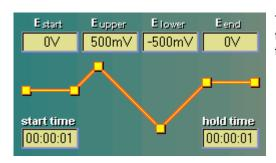
The duration of the starting phase and the final phase of the measurement are defined by the parameters 'start time' and 'end time'.
