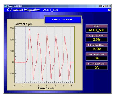
Calling up 'charge integration' results in an I(t) plot of the selected measurement. Five displays indicate the file name and the boundaries. An info box demands input of the interval of integration.
