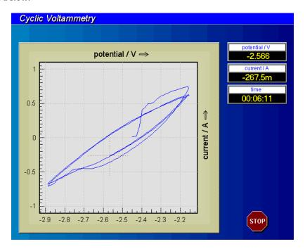
The measured U-I data is plotted online in the data window. At the upper right of the recording window three 'digital' instruments indicate the numeric values of the actually measured data triplett <U,I,t>. A running measurement can be terminated by using the <ESCAPE> function or by pressing the stop-button.
