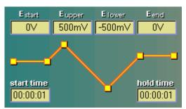
Four potentials can be defined independently. The 'start potential' offers the possibility to hold the probe at a certain potential before the cyclic part starts. 'Upper potential' and 'lower potential' define the upper and the lower reversing potentials. At the end of the measurement the potentiostat is fixed to the 'end potential'.
