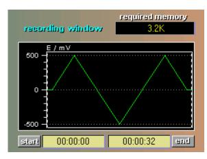
The function 'recording window' defines a time interval with active data acquisition. This interval covers the whole running time bas default setting. The window is defined by 'start' and 'end' margin. The use of the 'recording window' offers the
