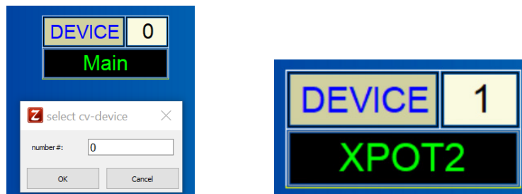
Fig. 5: Selecting an external potentiostat in test sampling window. DEVICE 1: XPOT2 indicates that the XPOT2 is connected to the port 1 of the EPC42 card.
