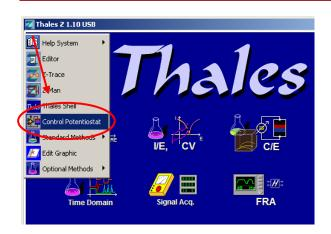
Click on the Z icon at the upper left edge of the Thales software window and switch to *Control Potentiostat* page.
