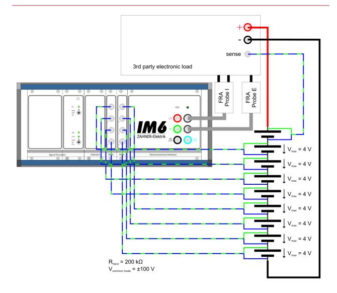
The PAD4 AD converter card is also compatible with a 3<sup>rd</sup> party electronic load interfaced from the ZENNIUM by means of the *FRA-Probe*.
