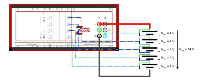
Connection scheme for 4 channel PAD4 with a 5 cell battery stack. The maximum input voltage of each PAD4 channel is limited to  $\pm 4$  V with a compliance voltage range of  $\pm 100$ V. The output voltage and current is limited by the electrochemical workstation. For example the *Zennium* has a compliance voltage of  $\pm 14$  V.
