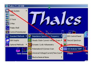
Click on the Z icon at the upper left edge of the Thales software window and navigate to *EIS Analysis "SIM"*.
