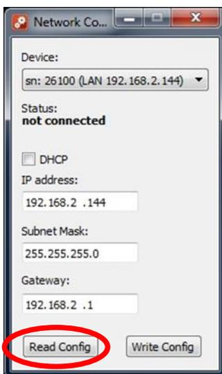
Before editing the IP settings press “Read Config” to load the current configuration. During read and write operations the status will show “connected”.
